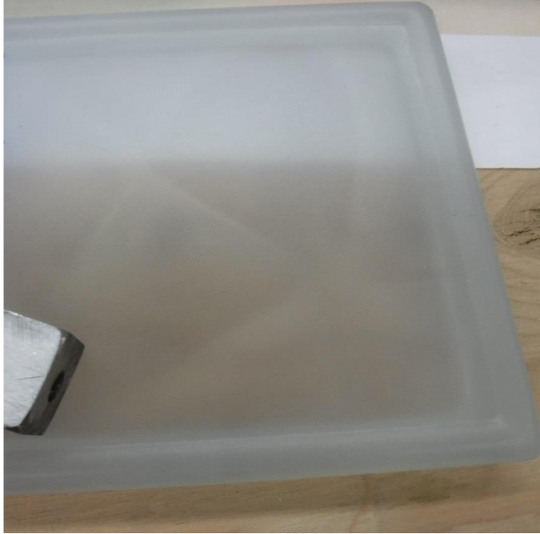
Photo No. 3 Method A: Un-Scored Surface After Cleaning
