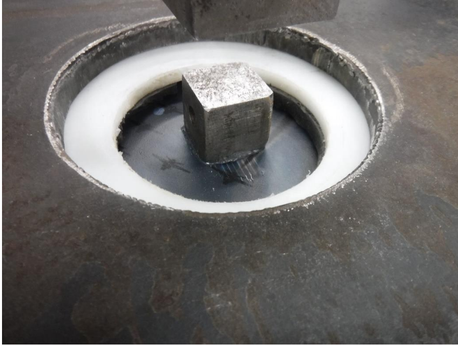
Photo No. 7 Steel Mounting Block Adhered to Surface
