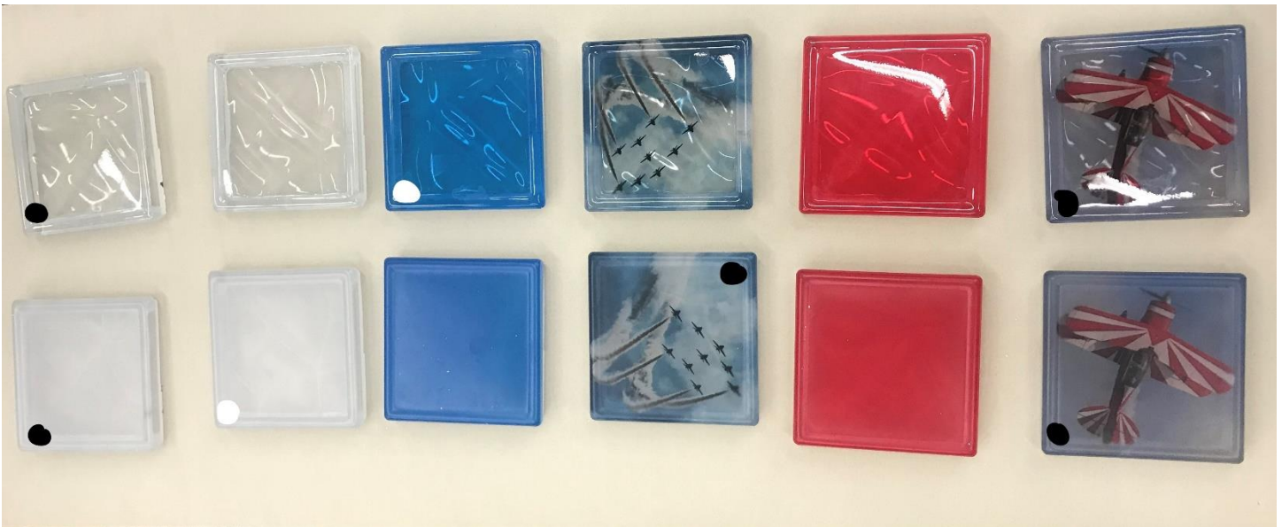
Photo No. 2 Materials Selected for Testing: Black Dot-Scored Surface, White Dot-Unscored Surface, No Dot: Not Tested
