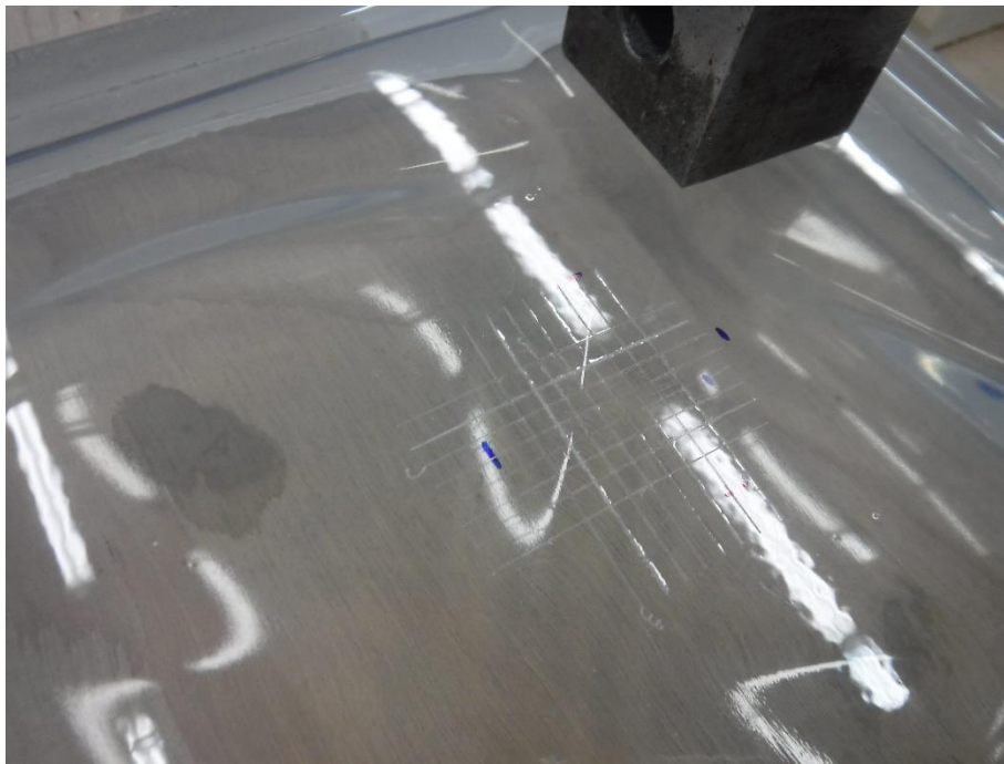
Photo No. 4 Method B: Scored Surface After Cleaning
