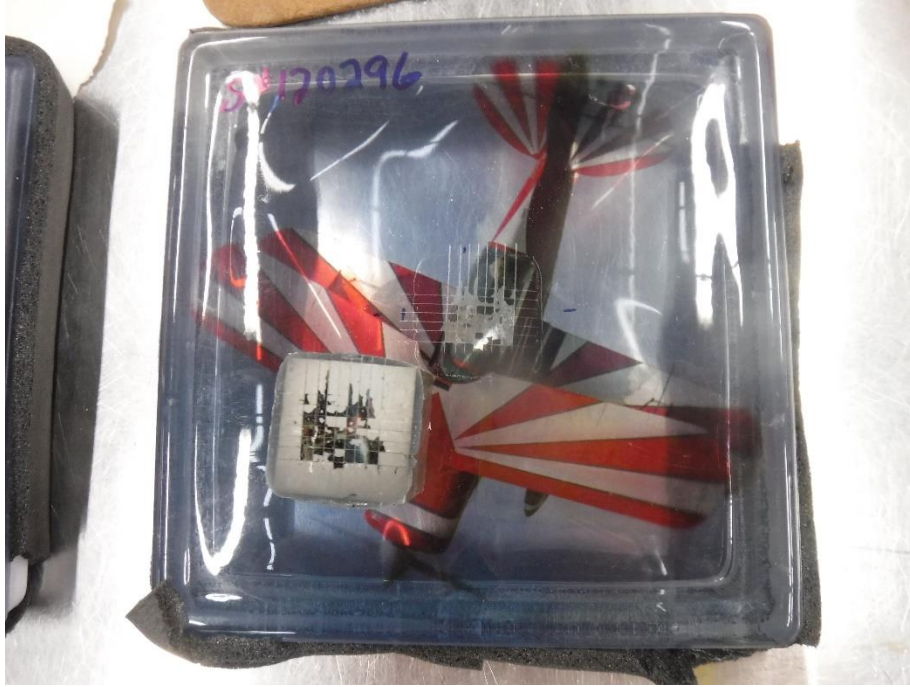
Photo No. 9 Mounting Block and Specimen After Pull Test
